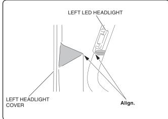
30. Install the assembled left headlight cover in the reverse order of removal.
