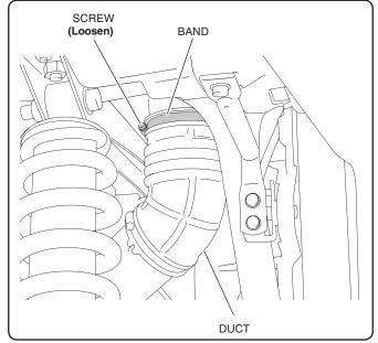
2. Remove the vehicle's parts as shown.
