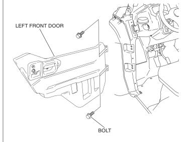
6. Remove the left front mudguard as shown.
