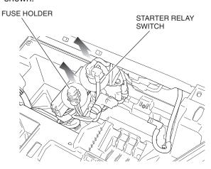
15. Remove the connectors as shown.
